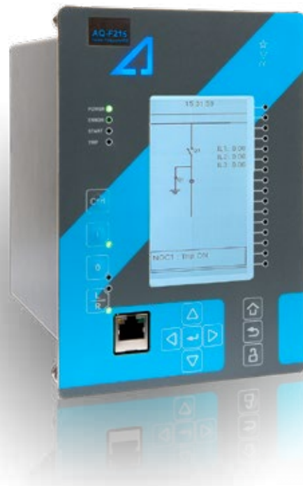
The AQ-F215 and AQ-F255 feeder terminal is equipped with the intermittent earth fault protection. The protection algorithm combined with 0.25 measurement class and 3.2 kHz sampling frequency, enables it to detect and isolate intermittent earth faults with high accuracy.
